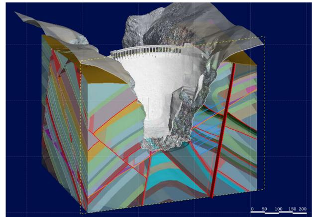
Figure 8. 3D screenshot of the combined structural and stratigraphic model of the LBD bedrock foundation. Different coloured layers represent individual unit contacts and discrete marker horizons. View looking NNE.
