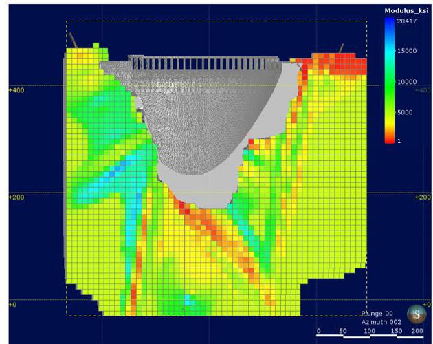
Figure 12. Example of a 2D vertical cross-section through an interpolated block model of rock mass deformation modulus values illustrating different rock strengths.
