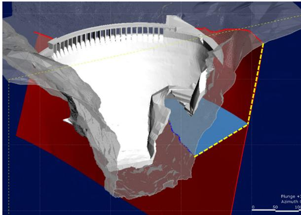
Figure 11. Example of a 2D vertical cross-section through the Baker River Canyon showing major shear zone SH2 (red) potentially forming a kinematically admissible plane shear block (yellow dash) with the Master Joint Set (blue) in the left abutment.
