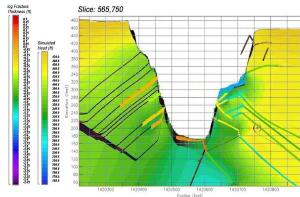
Figure 10. Example of a 2D vertical cross-section through the groundwater model showing the simulated heads with respect to the discrete fractures established through 3D modelling.
