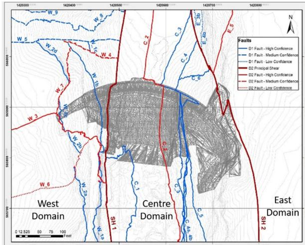
Figure 7. Plan map showing the surface expression of modelled faults and two principal shear zones (SH1 and SH2) that divide the area into three structural domains.
