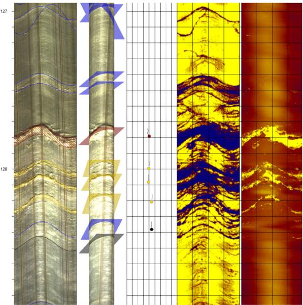
Figure 5. Example optical (left) and acoustic (right) televIEWER log from 2015 boring at LBD. 3D image (2<sup>nd</sup> from left) shows orientations of geologic structures as planes determined from the logging.
