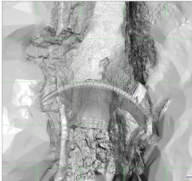
Figure 4. Plan view of LBD showing combined geospatial data (LiDAR and bathymetry). High-resolution DEM surfaces provide detail not achievable with aerial imagery.
