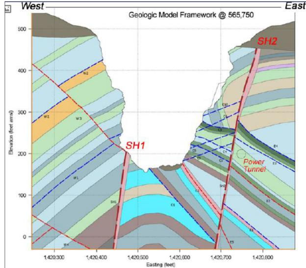
Figure 9. Example of a 2D vertical cross-section through the Baker River Canyon showing major faults (dashed red and blue) and lithological contacts.
